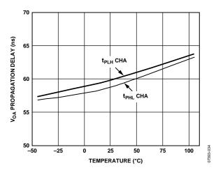
Figure 14. Typical Channel A Propagation Delay vs. Temperature
