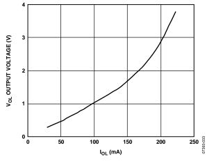
Figure 13. Typical  $V_{OL}$  vs.  $I_{OL}$  ( $V_{DD} = V_{DDL} = 5 \text{ V}$ ,  $V_{DDA} = V_{DDB} = 12 \text{ V}$  to 17 V)
