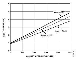
Figure 10. Typical  $I_{DDA}$  Supply Current,  $C_L = 200 pF$
