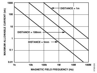
Figure 20. Maximum Allowable Current for Various Current-to-ADuM6132 Spacings
