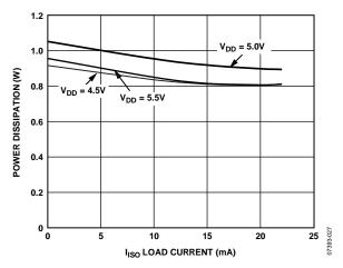
Figure 7. Typical Total Power Dissipation vs. I<sub>ISO</sub> External Load
