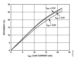
Figure 6. Typical V<sub>ISO</sub> Supply Efficiency vs. I<sub>ISO</sub> External Load
