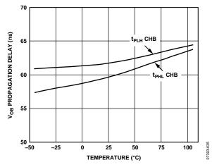
Figure 15. Typical Channel B Propagation Delay vs. Temperature
