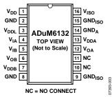
Figure 3. Pin Configuration
