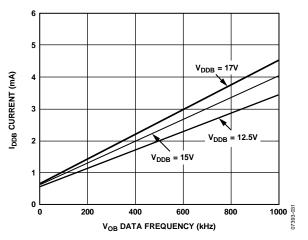
Figure 11. Typical  $I_{DDB}$  Supply Current,  $C_L = 200 pF$
