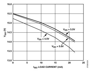
Figure 4. Typical V<sub>ISO</sub> Supply Voltage vs. I<sub>ISO</sub> External Load
