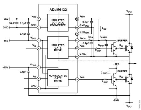
Figure 16. Typical Application Circuit
