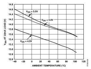
Figure 8. Typical V<sub>ISO</sub> Output Voltage at Maximum Combined Load over Temperature
