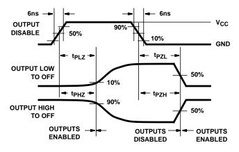
FIGURE 3. HC THREE-STATE PROPAGATION DELAY WAVEFORM
