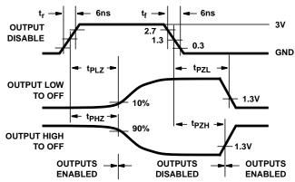
FIGURE 4. HCT THREE-STATE PROPAGATION DELAY WAVEFORM
