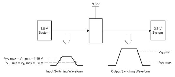
Figure 4. Switching Thresholds for 1.8-V to 3.3-V Translation
