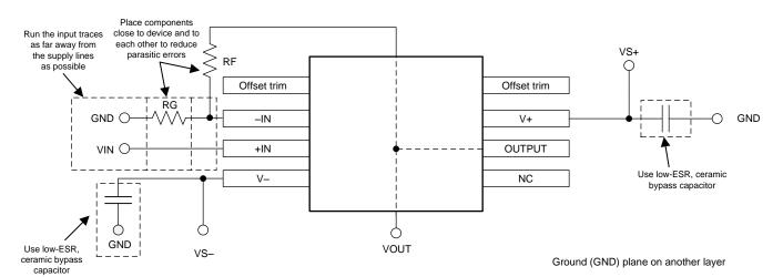
Figure 33. OPA277 Layout Example for the Noninverting Configuration
