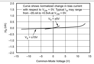
Figure 13. Change in Input Bias Current vs Power Supply Voltage
