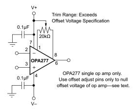
Figure 24. OPA277 Offset Voltage Trim Circuit
