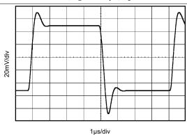
Figure 21. Small-Signal Step Response  $G=\pm 1$ ,  $C_L=0$ ,  $V_S=\pm 15$  V
