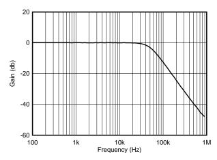
Figure 30. OPA277 Second-Order 50-kHz, Lowpass Filter
