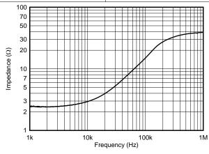
Figure 23. Open-Loop Output Impedance  $V_S = \pm 15 \text{ V}$
