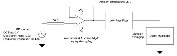
Figure 28. EMIRR IN+ Test Configuration Schematic
