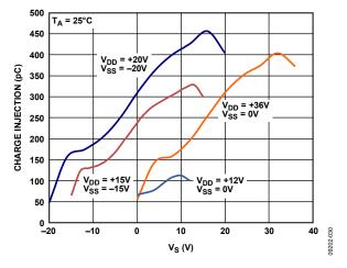
Figure 18. Charge Injection vs. Source Voltage
