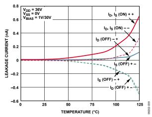
Figure 15. Leakage Currents vs. Temperature, 36 V Single Supply
