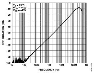
Figure 16. Off Isolation vs. Frequency, ±15 V Dual Supply
