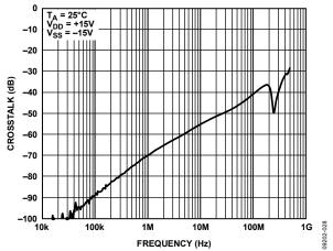
Figure 17. Crosstalk vs. Frequency, ±15 V Dual Supply
