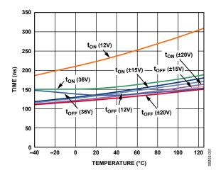
Figure 22.  $t_{ON}$ ,  $t_{OFF}$  Times vs. Temperature
