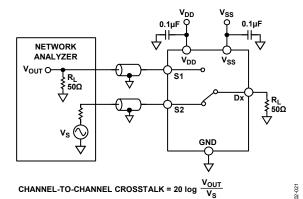
Figure 25. Channel-to-Channel Crosstalk
