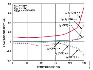
Figure 12. Leakage Currents vs. Temperature, ±15 V Dual Supply
