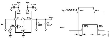
Figure 31. Switching Times
