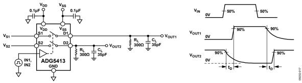
Figure 30. Break-Before-Make Time Delay, t<sub>D</sub>
