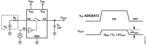
Figure 32. Charge Injection
