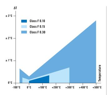
Tolerances of base values for Pt temperature sensors are specified in DIN EN 60751.
