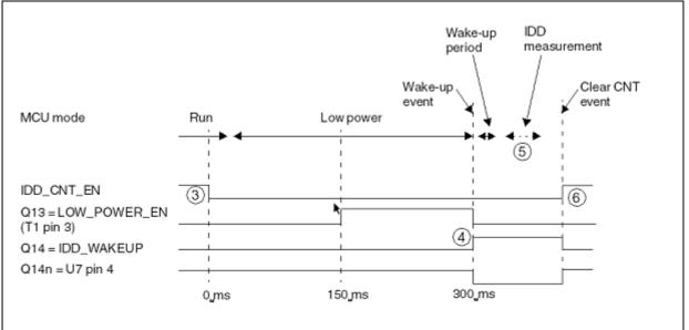
The Low power mode measurement procedure can be used in Halt or Active halt mode if the  $I_{DD}$  current does not exceed 30 uA, otherwise the  $I_{DD}$  measurement procedure in Run mode should be used up to 30 mA.
