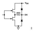
Figure 9. Digital Output Stage
