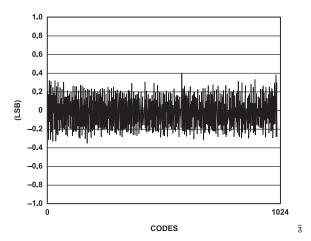
Figure 41. Typical DNL Plot, 10.3 MHz A<sub>IN</sub> @ 80 MSPS
