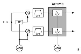
Figure 44. Typical I/Q Demodulation Scheme
