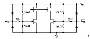
Figure 6. Analog Input Stage
