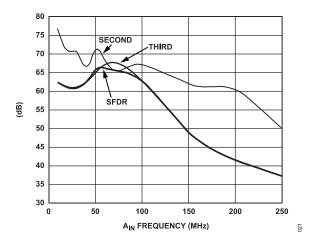
Figure 21. Harmonic Distortion (Second and Third) and SFDR vs. A<sub>IN</sub> Frequency (1 V p-p, FS = 105 MSPS)
