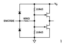
Figure 7. Encode Inputs
