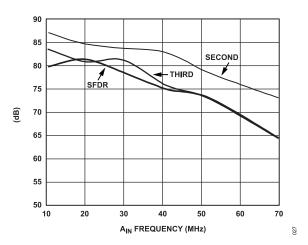
Figure 27. Harmonic Distortion (Second and Third) and SFDR vs. A<sub>IN</sub> Frequency (1 V p-p, FS = 40 MSPS)
