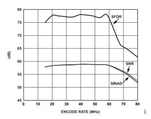
Figure 31. SINAD and SFDR vs. Encode Rate ( $A_{\rm IN}$  = 10.3 MHz, 65 MSPS Grade)  $A_{\rm IN}$  = -0.5 dBFS Differential, 1 V p-p Analog Input Range
