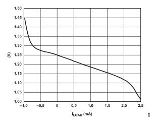
Figure 38.  $V_{REF}$  vs.  $I_{LOAD}$
