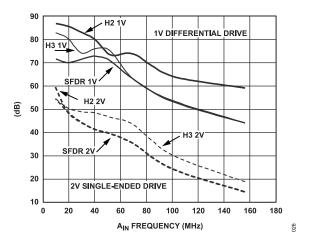
Figure 26. Harmonic Distortion (Second and Third) and SFDR vs. A<sub>IN</sub> Frequency (FS = 65 MSPS)
