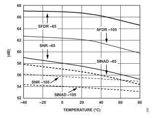
Figure 37. SNR, SINAD, SFDR vs. Temperature,  $A_{\rm IN}$  = 10.3 MHz, -65 MSPS Grade, -105 MSPS Grade, 1 V p-p
