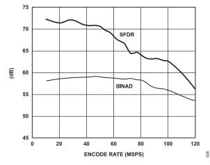
Figure 28. SINAD and SFDR vs. Encode Rate ( $A_{\rm IN}$  = 10.3 MHz, 105 MSPS Grade,  $A_{\rm IN}$  = -0.5 dBFS Differential, 1 V p-p Analog Input Range)
