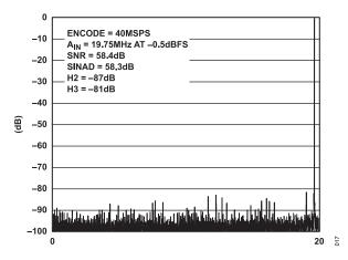
Figure 17. FFT: FS = 40 MSPS,  $A_{\rm IN}$  = 19.75 MHz @ -0.5 dBFS, Differential, 1 V p-p Input Range
