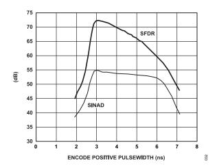
Figure 32. SINAD and SFDR vs. Encode Pulse Width High,  $A_{\rm IN}$  = -0.5 dBFS Single-Ended, 1 V p-p Analog Input Range 105 MSPS
