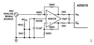
Figure 43. Using the AD8138 to Drive the AD9218
