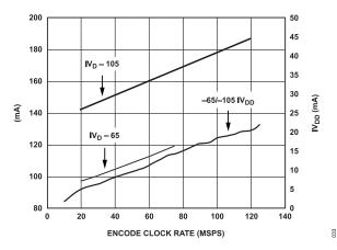
Figure 33. IV $_{\rm D}$  and IV $_{\rm DD}$  vs. Encode Rate (A $_{\rm IN}$  = 10.3 MHz, @ -0.5 dBFS), -65 MSPS/-105 MSPS Grade CI = 5 pF
