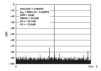
Figure 23. FFT: FS = 31 MSPS, A<sub>IN</sub> = 8 MHz @ -0.5 dBFS, Differential, with AD8138 Driving ADC Inputs,1 V p-p Input Range
