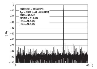
Figure 18. FFT: FS = 105 MSPS,  $A_{IN}$  = 70 MHz @ -0.5 dBFS, Differential, 1 V p-p Input Range
