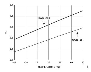
Figure 36. Gain Error vs. Temperature,  $A_{\rm IN}$  = 10.3 MHz, -65 MSPS Grade, -105 MSPS Grade, 1 V p-p
