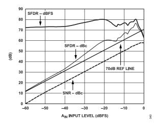
Figure 40. SFDR vs. A<sub>IN</sub> Input Level, 10.3 MHz A<sub>IN</sub> @ 80 MSPS
