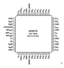
Figure 5. Pin Configuration
