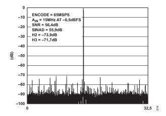
Figure 19. FFT: FS = 65 MSPS,  $A_{IN}$  = 15 MHz @ - 0.5 dBFS; with AD8138 Driving ADC Inputs, 1 V p-p Input Range
