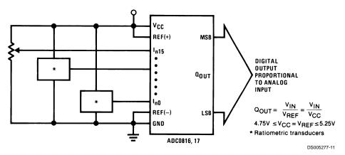
FIGURE 9. Ratiometric Conversion System
