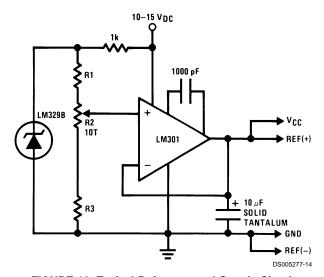
FIGURE 12. Typical Reference and Supply Circuit
