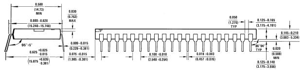
Molded Dual-In-Line Package (N) **NS Package Number N40A**
