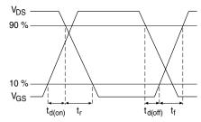
Fig. 10b - Switching Time Waveforms
