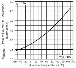
Fig. 4 - Normalized On-Resistance vs. Temperature
