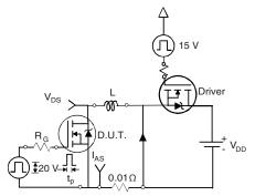
Fig. 12a - Unclamped Inductive Test Circuit
