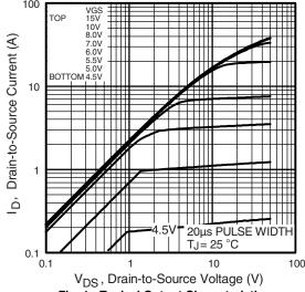
Fig. 1 - Typical Output Characteristics
