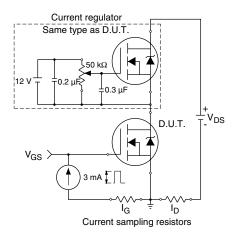
Fig. 13b - Gate Charge Test Circuit
