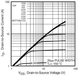
Fig. 2 - Typical Output Characteristics
