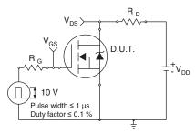
Fig. 10a - Switching Time Test Circuit
