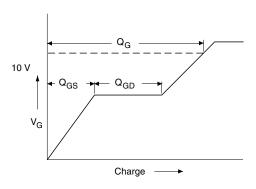
Fig. 13a - Basic Gate Charge Waveform
