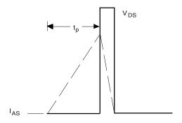
Fig. 12b - Unclamped Inductive Waveforms
