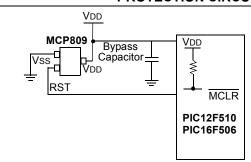
Note: This brown-out protection circuit employs Microchip Technology's MCP809 microcontroller supervisor. There are 7 different trip point selections to accommodate 5V to 3V systems.
