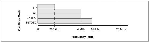
FIGURE 13-3: VOLTAGE FREQUENCY GRAPH, -40°C ≤ TA ≤ +125°C (PIC16F506)
