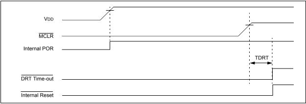
FIGURE 10-9: TIME-OUT SEQUENCE ON POWER-UP (MCLR TIED TO VDD): FAST VDD RISE TIME
