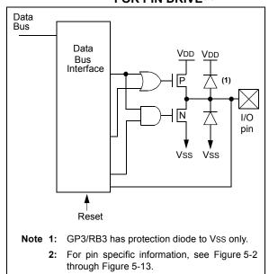
FIGURE 5-2: BLOCK DIAGRAM OF GP0/RB0 AND GP1/RB1
