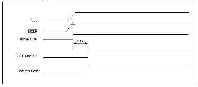
FIGURE 10-10: TIME-OUT SEQUENCE ON POWER-UP (MCLR TIED TO VDD): SLOW VDD RISE TIME
