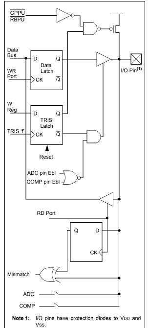
FIGURE 5-3: BLOCK DIAGRAM OF GP3/RB3 (With Weak Pull-up And Wake-up On
