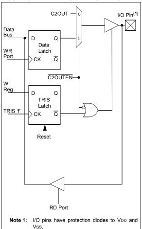
FIGURE 5-13: BLOCK DIAGRAM OF RC5
