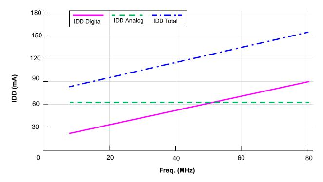
Figure 3-1 Maximum Run IDD vs. Frequency (see Note 6. in Figure 3-14)
