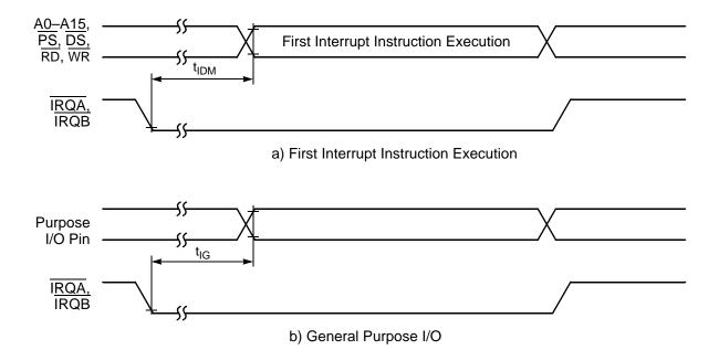
Figure 3-14 External Level-Sensitive Interrupt Timing
