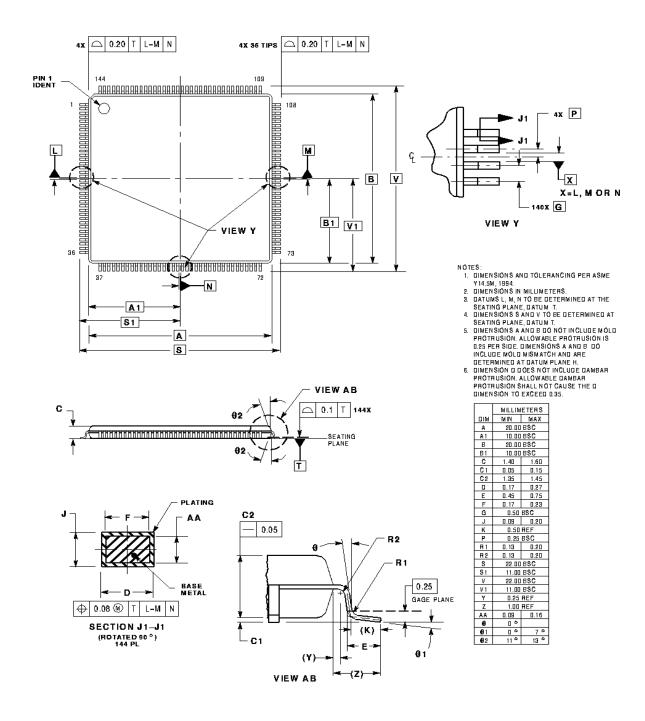
Figure 4-2 144-pin LQFP Mechanical Information
