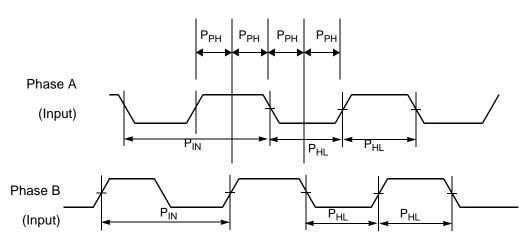
**Figure 3-24 Quadrature Decoder Timing**
