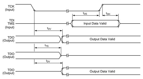
Figure 3-30 Test Access Port Timing Diagram
