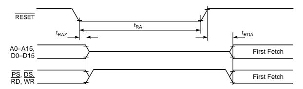
**Figure 3-12 Asynchronous Reset Timing**
