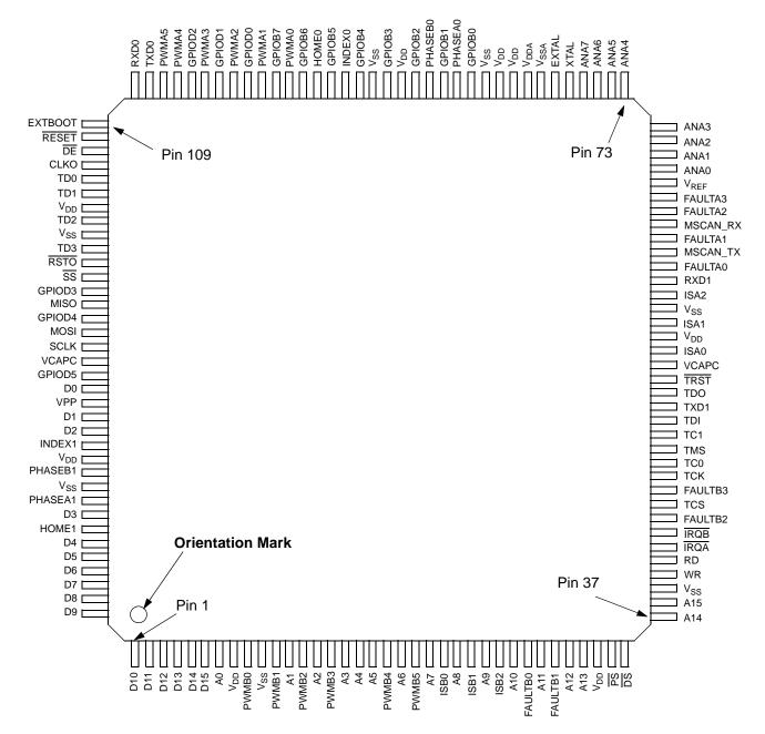
Figure 4-1 Top View, 56F805 144-pin LQFP Package
