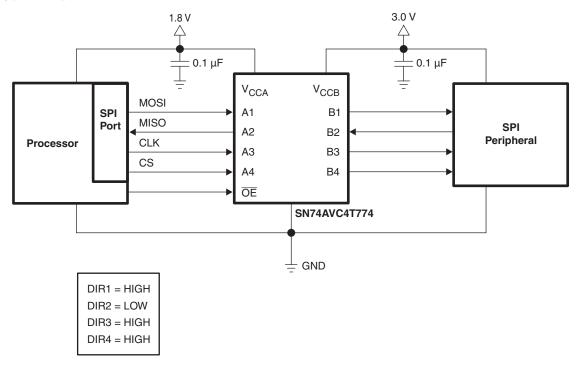
Figure 5. Typical Application of the SN74AVC4T774
