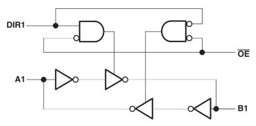
Figure 4. Logic Diagram (Positive Logic)
