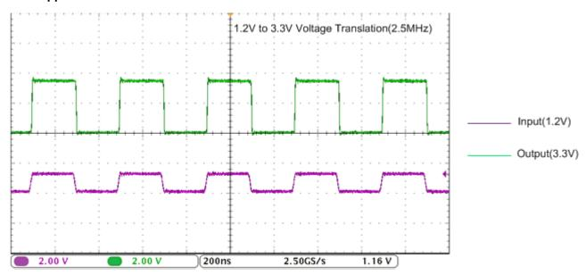
Figure 6. Translation Up (1.2 V to 3.3 V) at 2.5 MHz
