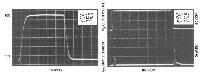
Figure 12. Drive Output Waveform
