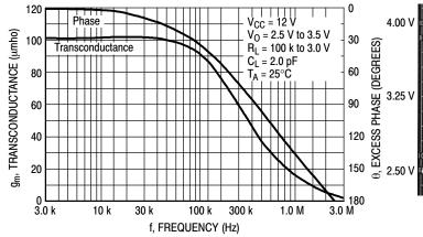
Figure 6. Error Amp Transconductance and Phase versus Frequency
