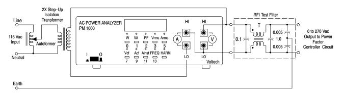
Figure 25. Power Factor Test Set-Up
