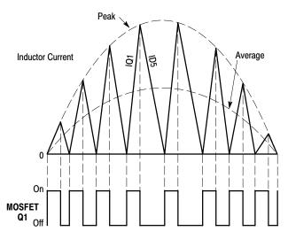
Figure 19. Inductor Current and MOSFET Gate Voltage Waveforms
