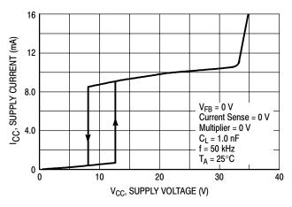
Figure 14. Supply Current versus Supply Voltage
