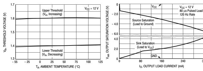
Figure 10. Zero Current Detector Input Threshold Voltage versus Temperature
