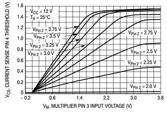
Figure 2. Current Sense Input Threshold versus Multiplier Input
