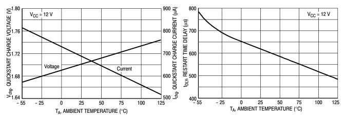
Figure 8. Quickstart Charge Current versus Temperature
