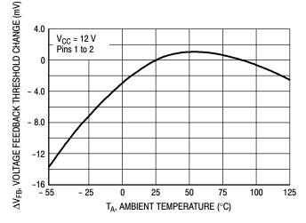
Figure 4. Voltage Feedback Input Threshold Change versus Temperature
