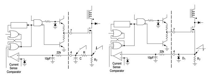
Figure 27. Current Waveform Spike Suppression
