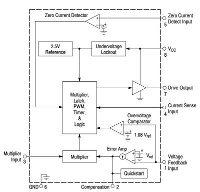
Figure 1. Simplified Block Diagram
