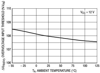
Figure 5. Overvoltage Comparator Input Threshold versus Temperature
