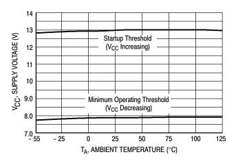
Figure 15. Undervoltage Lockout Thresholds versus Temperature
