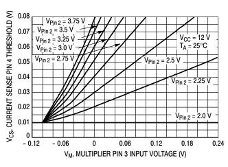
Figure 3. Current Sense Input Threshold versus Multiplier Input, Expanded View
