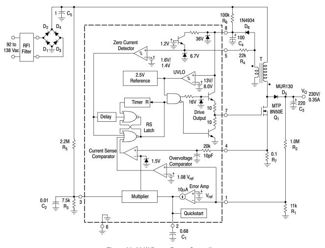
Figure 20. 80 W Power Factor Controller
