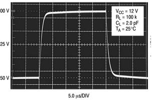
Figure 7. Error Amp Transient Response
