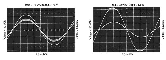
Figure 23. Power Factor Corrected Input Waveforms (Figure 20 Circuit)
