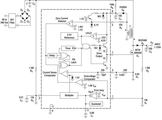
Figure 22. 450 W Universal Input Power Factor Controller
