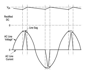
Figure 17. Uncorrected Power Factor Input Waveforms
