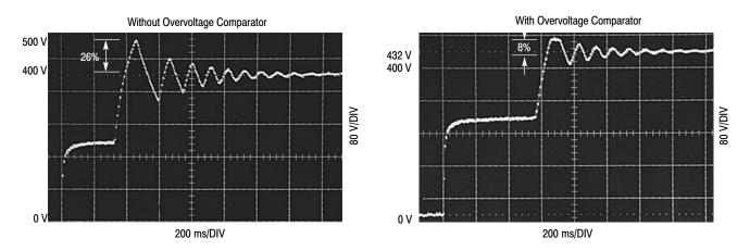
Figure 24. Output Voltage Startup Overshoot (Figure 20 Circuit)
