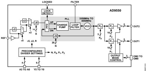
Figure 23. Detailed Block Diagram
