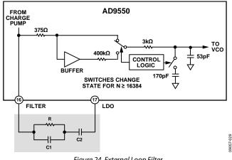
Figure 24. External Loop Filter
