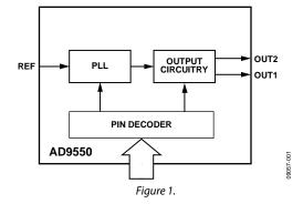
15 possible input frequencies to a list of 52 possible output frequency pairs (OUT1 and OUT2).
