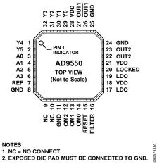
Figure 2. Pin Configuration
