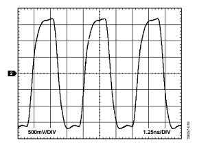
Figure 20. Typical Output Waveform, CMOS (250 MHz, 10 pF Load)
