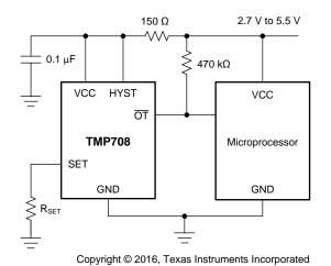
Figure 5. Overtemperature Protection for a 60°C Trip Point
