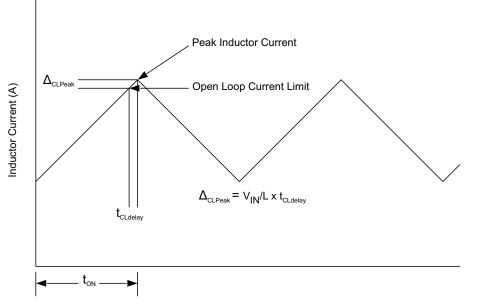
Figure 23. Current Limit Delay
