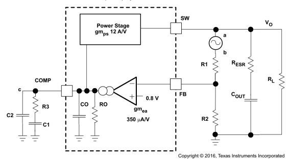
Figure 28. Small Signal Model for Loop Response
