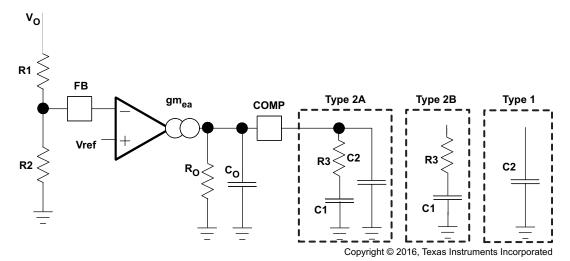
Figure 30. Types of Frequency Compensation
