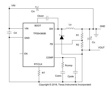
Figure 50. TPS54360B Inverting Power Supply
