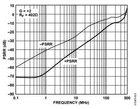
Figure 21. PSRR vs. Frequency
