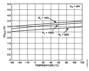
Figure 30. Output Swing vs. Temperature
