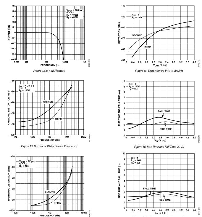
Figure 17. Rise Time and Fall Time vs. V<sub>IN</sub>
