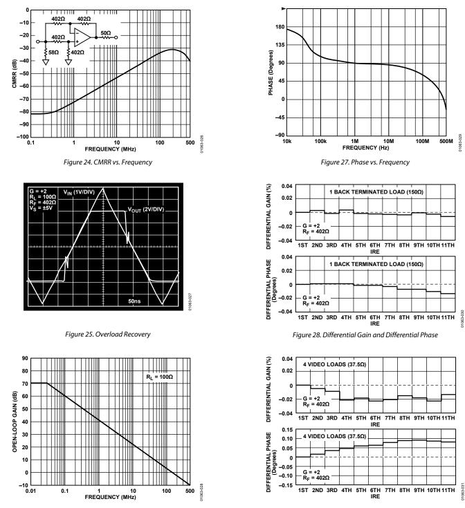
Figure 26. Open-Loop Gain vs. Frequency
