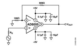
Figure 38. Low Noise, Low Power Preamp with G = +10 and BW = 20 MHz
