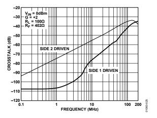
Figure 23. Crosstalk (Output-to-Output) vs. Frequency
