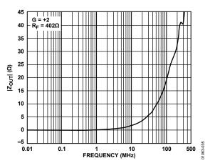
Figure 33. Output Impedance vs. Frequency
