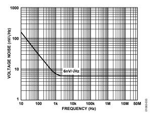
Figure 31. Voltage Noise vs. Frequency
