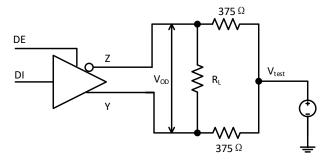
Figure 8-1. Driver Differential Output Voltage With Common-Mode Load
