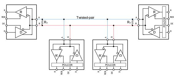
Figure 10-1. Typical RS-485 Network With CA-IF48xxHS/HM/HD Half-Duplex Transceivers
