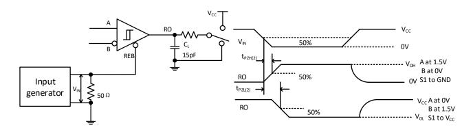
Figure 8-8. Receiver Enable Times With Driver Disabled
