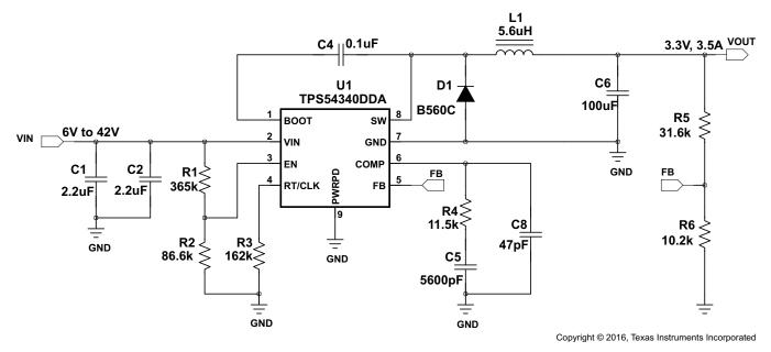
Figure 32. 3.3 V Output TPS54340 Design Example
