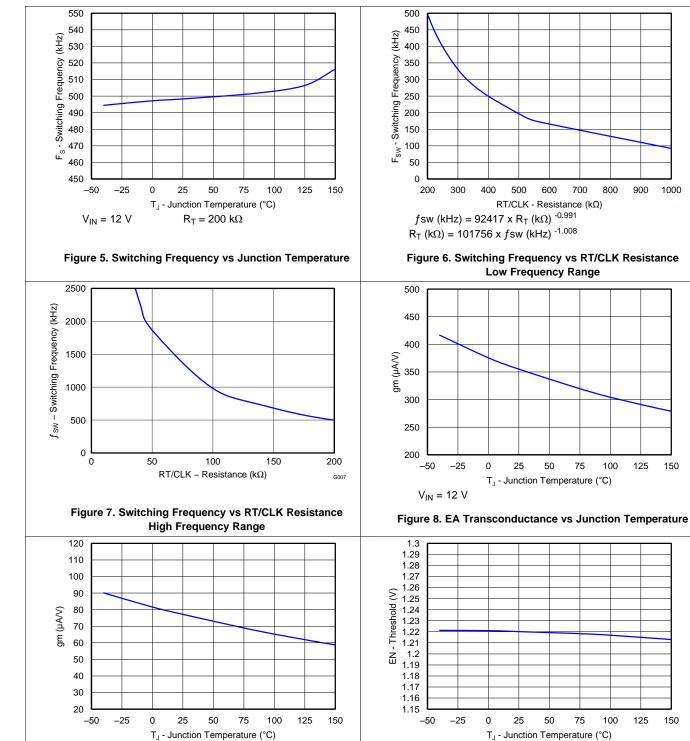
Figure 10. EN Terminal Voltage vs Junction Temperature
