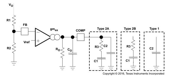
Figure 30. Types of Frequency Compensation
