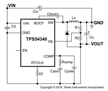
Figure 50. TPS54340 Inverting Power Supply
