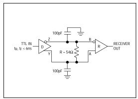
Figure 10. Receiver Propagation-Delay Test Circuit
