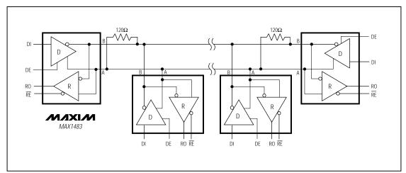
Figure 14. MAX1483 Typical Half-Duplex RS-485 Network
