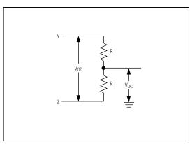
Figure 1. Driver DC Test Load
