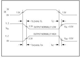
Figure 6. Driver Enable and Disable Times
