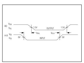
Figure 7. Receiver Propagation Delays
