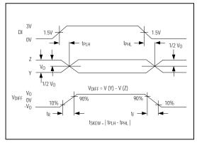
Figure 5. Driver Propagation Delays
