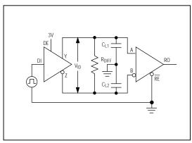
Figure 3. Driver/Receiver Timing Test Circuit
