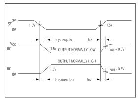
Figure 8. Receiver Enable and Disable Times
