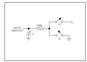
Figure 4. Driver Timing Test Load
