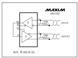
Figure 16. Line Repeater for MAX1482
