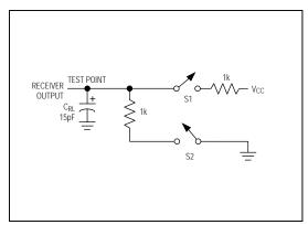
Figure 2. Receiver Timing Test Load
