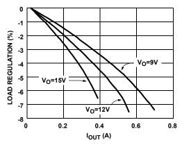
FIGURE 7.  $V_{\mbox{\footnotesize{BOOST}}}$  LOAD REGULATION AT  $V_{\mbox{\footnotesize{IN}}}$ =3V (P MODE)
