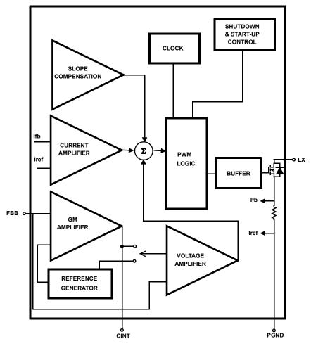
FIGURE 19. BLOCK DIAGRAM OF THE BOOST REGULATOR
