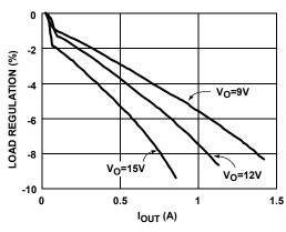
FIGURE 8.  $V_{BOOST}$  LOAD REGULATION AT  $V_{IN}$ =5V (P MODE)
