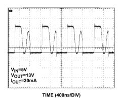
FIGURE 16. LX WAVEFORM - DISCONTINUOUS MODE
