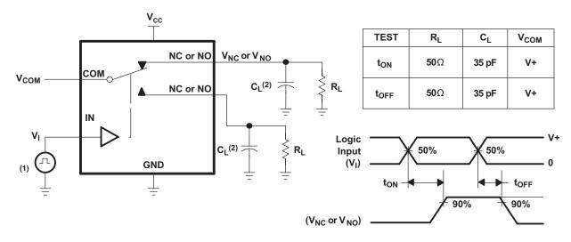
A. All input pulses are supplied by generators having the following characteristics: PRR ≤ 10 MHz,  $Z_0$  = 50  $\Omega$ ,  $t_r$  < 5 ns,  $t_f$  < 5 ns.
