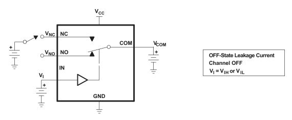
Figure 17. OFF-State Leakage Current (I<sub>NC(OFF)</sub>, I<sub>NC(PWROFF)</sub>, I<sub>NO(OFF)</sub>, I<sub>NO(PWROFF)</sub>, I<sub>COM(OFF)</sub>, I<sub>COM(PWROFF)</sub>)
