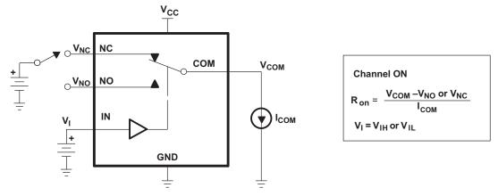
Figure 16. ON-state Resistance (R<sub>ON</sub>)
