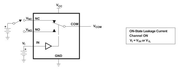
Figure 18. ON-State Leakage Current (I<sub>COM(ON)</sub>, I<sub>NC(ON)</sub>, I<sub>NO(ON)</sub>)
