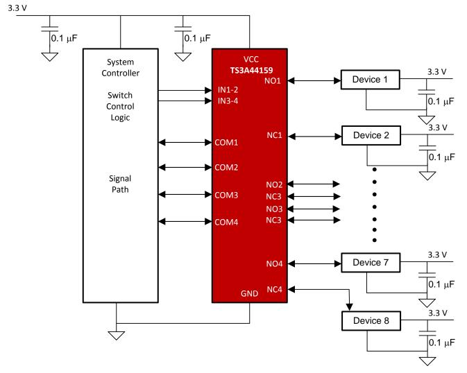
Figure 28. Typical Application Diagram
