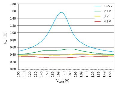
Figure 29. R<sub>on</sub> vs V<sub>COM</sub> (All Voltages)
