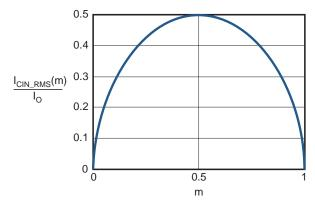
Figure 2. I<sub>CIN</sub> vs. Voltage Conversion Ratio
