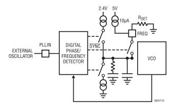
Figure 16. Phase-Locked Loop Block Diagram
