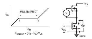
Figure 9. Gate Charge Characteristic
