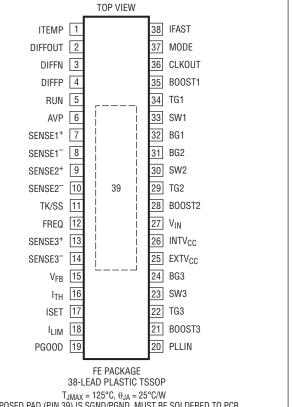
$T_{JMAX} = 125^{\circ}C, \; \theta_{JA} = 25^{\circ}CW$  EXPOSED PAD (PIN 39) IS SGND/PGND, MUST BE SOLDERED TO PCB
