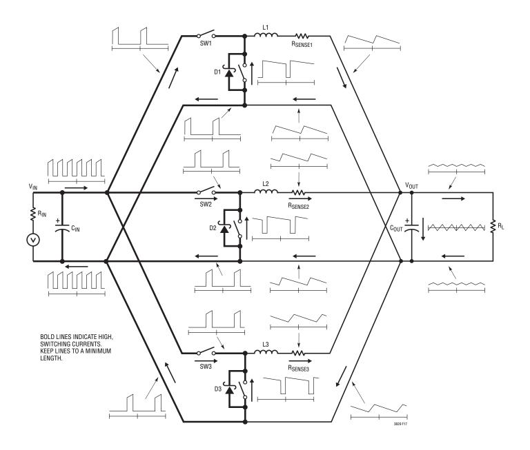
Figure 17. Branch Current Waveform
