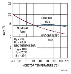
Figure 6. Worst-Case I<sub>MAX</sub> Versus Inductor Temperature Curve with and without NTC Temperature Compensation
