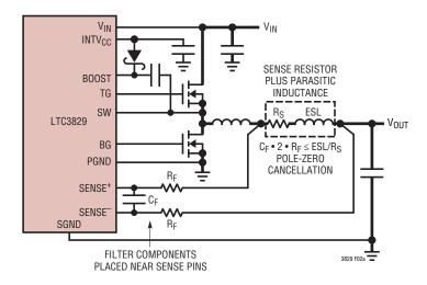
(2a) Using a Resistor to Sense Current
