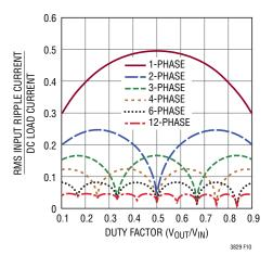
Figure 10. Normalized Input RMS Ripple Current vs Duty Factor for One to Six Output Stages
