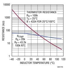
Figure 5. Resistance Versus Temperature for the ITEMP Pin Network and the 100k NTC
