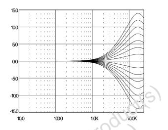
Figure 18. Treble Center Frequencies @ Gain = 14dB
