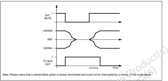
For timing purposes the Bit 3 of the I<sup>2</sup>C bus output register is set to 1 ron, the start of muting until the end of demuting.
