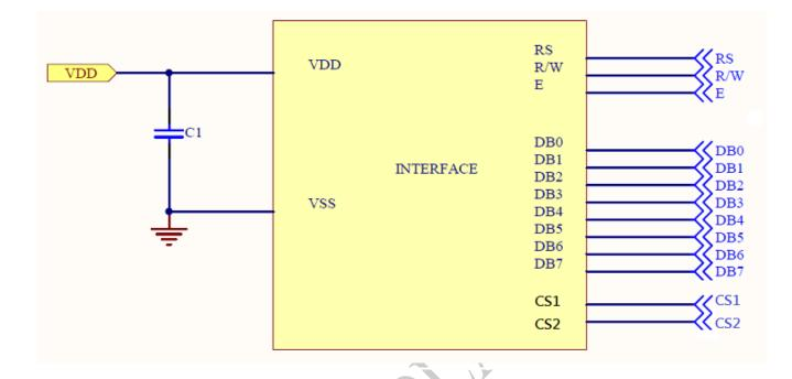
Pin connected to MCU interface: RS, R/W, E, DB0~7,CS1,CS2
