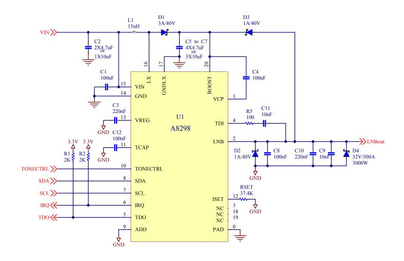
Schematic 2. DiSEqC 1.0 Applications, 12 V  $_{IN}$  ±10%, 700 mA I  $_{OUT},$  surge of ±1000 V, 2  $\Omega,$  1.2/50  $\mu s-8/20$   $\mu s$  combination wave
