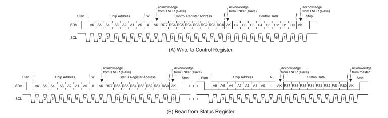
Figure 8. I<sup>2</sup>C™ Interface Read and Write Sequences. (A) for the I<sup>2</sup>C™ Write cycle and (B) for the I<sup>2</sup>C™ Read cycle
