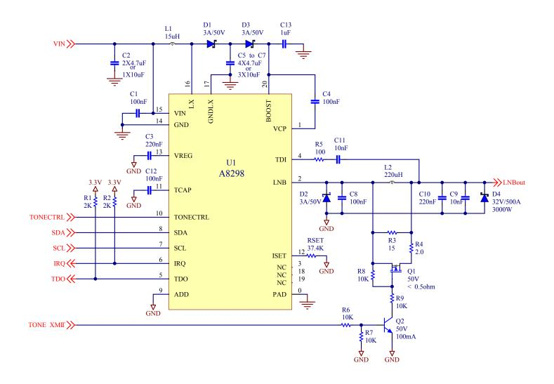
Schematic 3. DiSEqC 2.0 Applications for increased surge requirements  $\pm 1000$  V, 2  $\Omega,$  1.2/50  $\mu s-8/20$   $\mu s$  combination wave, and "stress to TVS failure" (or  $\pm 4000$  V) test
