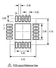
For Reference Only (reference JEDEC MO-220WGGD) Dimensions in millimeters
