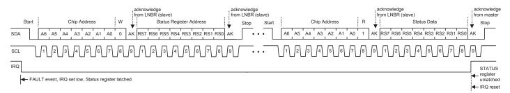
Figure 9. Fault, IRQ, and Status Register Timing. When a UVLO, OCP, or TSD event occurs, the IRQ bit is set low and the Status register is latched. The IRQ bit is reset to high when the A8298 acknowledges it is being read. The Status register is unlatched when the master acknowledges the status data from the A8298.
