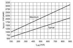
Figure 4. Boost inductor peak current versus  $I_{LNB}$  for the A8298
