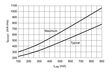
Figure 6. Boost capacitor rms current versus  $I_{\text{LNB}}$  for the A8298
