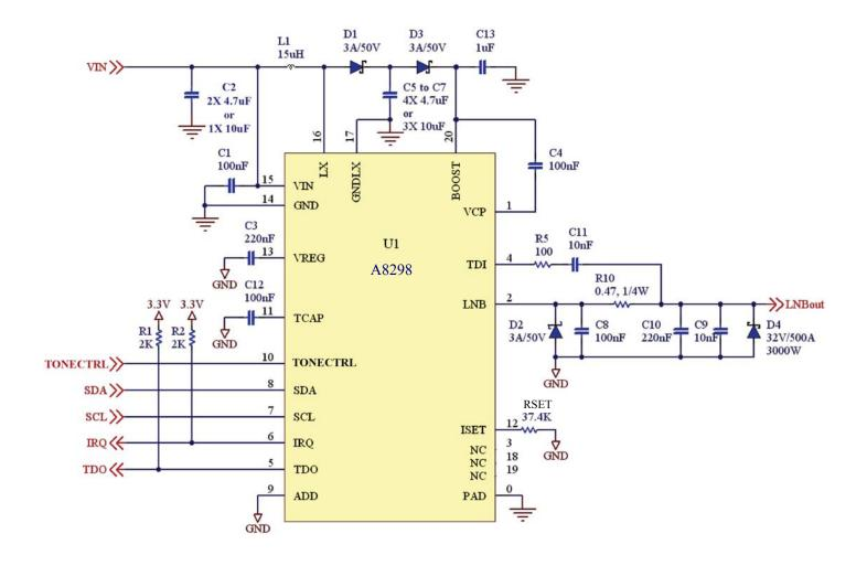
Schematic 4. DiSEqC 1.0 Applications for increased surge requirements  $\pm 1000$  V, 2  $\Omega$ , 1.2/50  $\mu$ s – 8/20  $\mu$ s combination wave, and "stress to TVS failure" (or  $\pm 4000$  V) test
