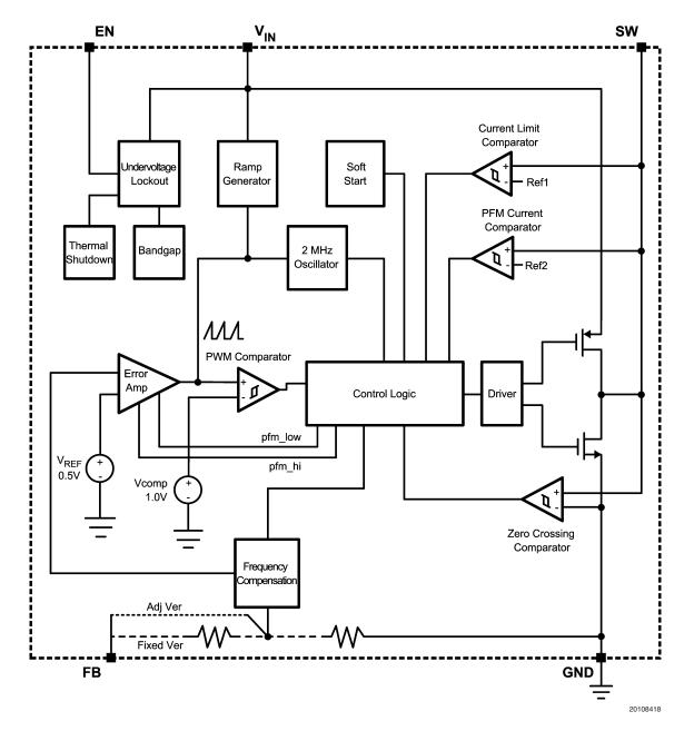
FIGURE 4. Simplified Functional Diagram
