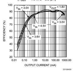
Efficiency vs. Output Current (V<sub>OUT</sub> = 3.3V, L= 2.2 μH)
