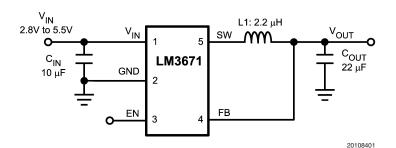
FIGURE 1. Typical Application Circuit
