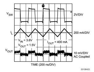
FIGURE 5. Typical PWM Operation
