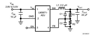
FIGURE 2. Typical Application Circuit for ADJ version
