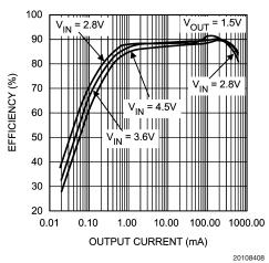
Efficiency vs. Output Current (V<sub>OUT</sub> = 2.5V, L= 2.2 μH)
