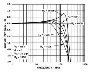
Figure 7. Bandwidth vs. Feedback Resistor—Dual Supply
