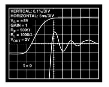
Figure 18. Settling Time
