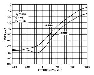
Figure 13. PSRR vs. Frequency
