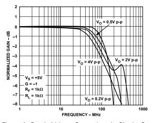
Figure 6. Bandwidth vs. Output Level—Single Supply, Gain of –1
