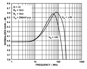
Figure 9. Gain Flatness—Small Signal
