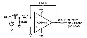
Figure 21. AD8014 as a Photodiode Preamp
