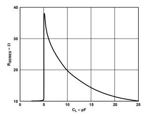
Figure 26. Driving Capacitive Load
