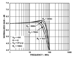
Figure 8. Bandwidth vs. Feedback Resistor—Single Supply
