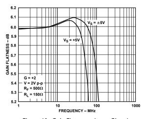
Figure 10. Gain Flatness—Large Signal
