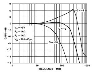
Figure 12. Bandwidth vs. Gain—Single Supply
