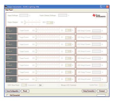
2. Click "Setup Connection" on the GUI and ensure the Baud Rate is set to 57600 and that the "Boot on Connect" box is unchecked.
