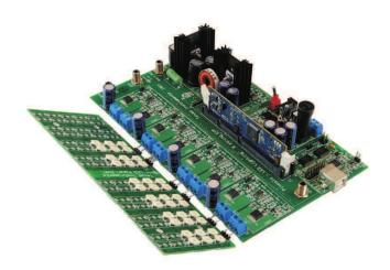
This document provides instructions to run a GUI that controls the DC/DC LED Lighting Developer's Kit board using the Piccolo F28035 microcontroller.
