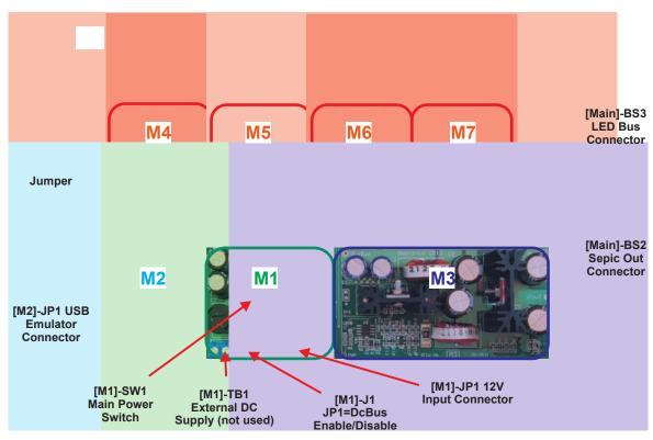
Step 1. On the Piccolo F28035 controlCARD, check the following switches:
