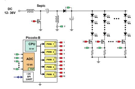
A typical power conversion board is made up of several power stages. On the Lighting\_DCDC board, each of these power stages takes the form of a macro section. Each of these macro sections is bounded by its own silkscreen area. Below is a list of all the macro blocks' names and a short description of their functions. Refer to the image on the next page for placement of macro areas.
