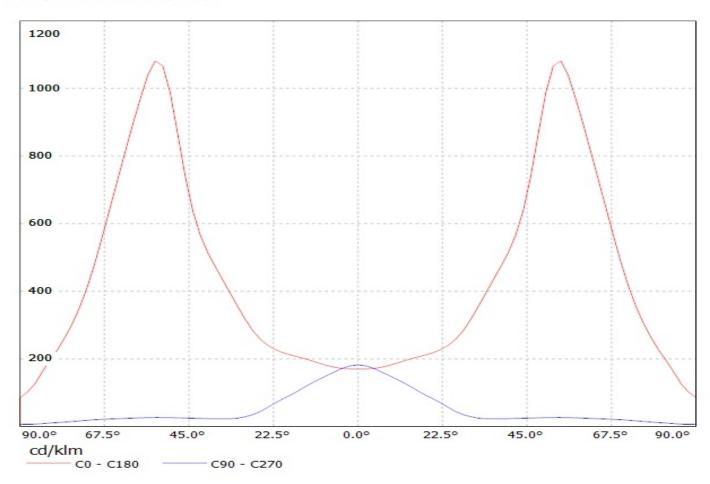
Luminaire: Ledil Oy C10818\_Strada-A-XPG C10818\_Strada-A-XPG Lamps: 1 x Cree XP-G (White)
