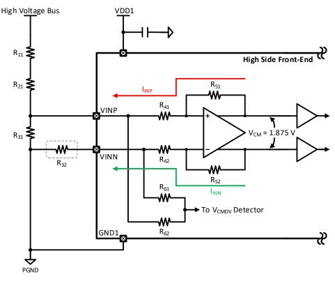
Figure 9-2. Typical Application Circuit for Voltage-Measurement
