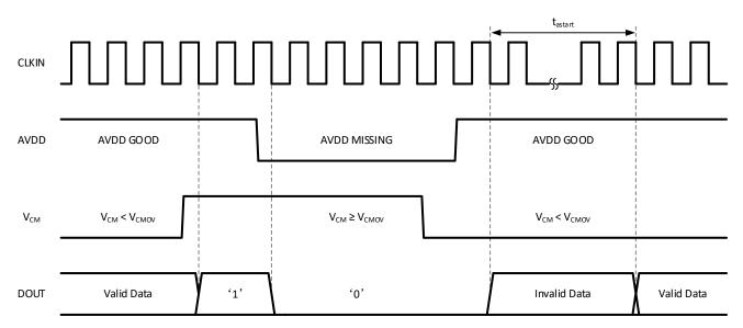
Figure 8-5. CA-IS1305x Over-range Output Waveforms
