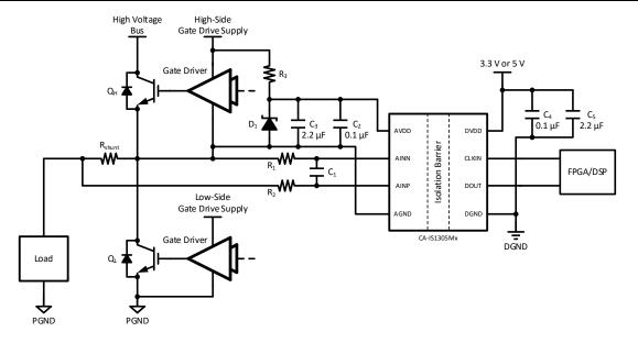
Figure 9-1. Typical Application for 1-phase Current Sensing
