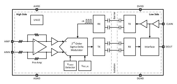
Figure 8-1. Functional Block Diagram of the CA-IS1305x
