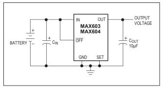
Figure 6. 3.3V or 5V Linear-Regulator Application
