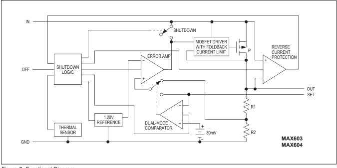
Figure 2. Functional Diagram
