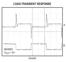
A: OUTPUT VOLTAGE (100mV/div) B: I<sub>OUT</sub> = 500mA (HIGH), I<sub>OUT</sub> = 5mA (LOW)
