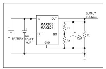
Figure 3. Adjustable Output Using External Feedback Resistors
