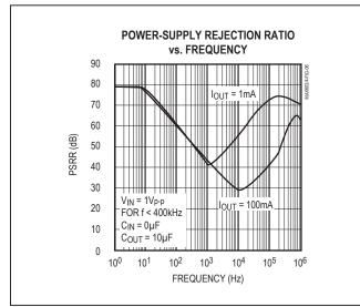
Figure 7. Power-Supply Rejection Ratio vs. Ripple Frequency
