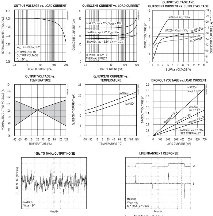
A:  $V_{IN}$  = 8V (HIGH),  $V_{IN}$  = 7V (LOW) B: OUTPUT VOLTAGE (50mV/div)
