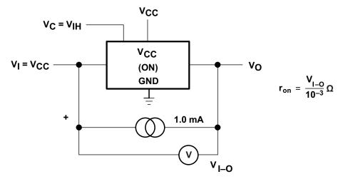
Figure 2. ON-State Resistance Test Circuit
