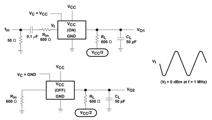
Figure 10. Crosstalk Between Any Two Switches
