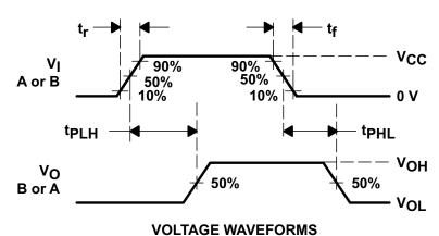
Figure 5. Propagation Delay Time, Signal Input to Signal Output
