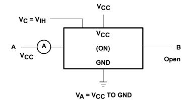
Figure 4. ON-State Leakage-Current Test Circuit
