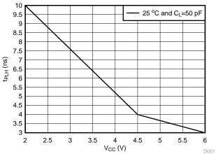
Figure 1.  $t_{PLH}$  vs  $V_{CC}$
