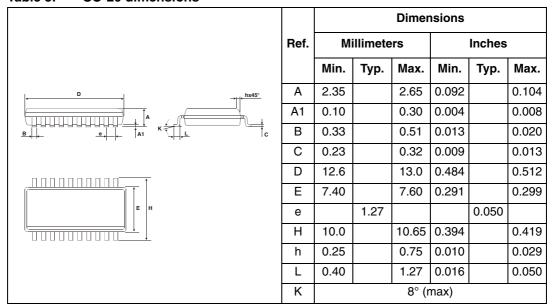
Figure 11. SO-20 footprint (dimensions in mm)
