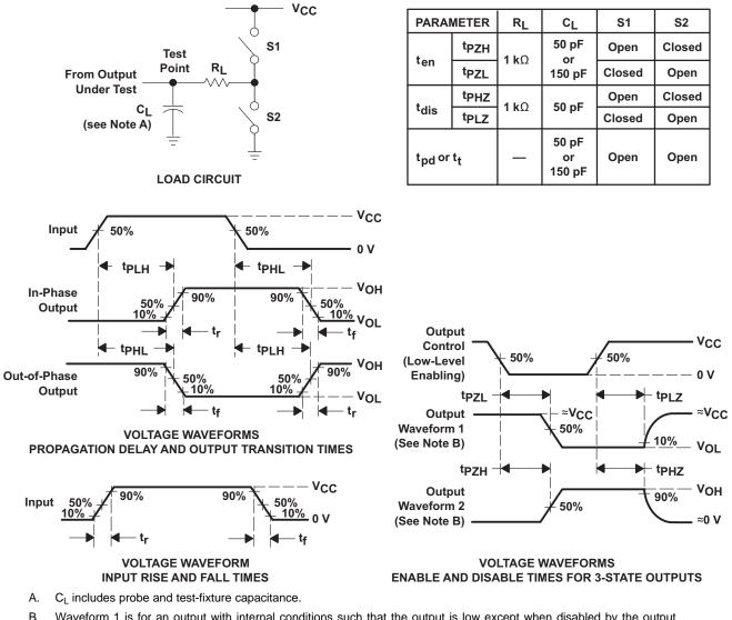
B. Waveform 1 is for an output with internal conditions such that the output is low except when disabled by the output control.
