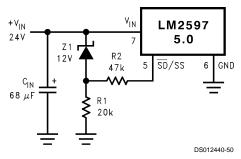
FIGURE 31. Undervoltage Lockout for a Buck Regulator
