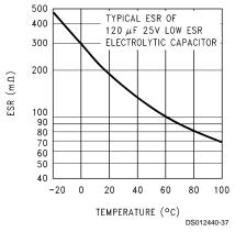
FIGURE 18. Capacitor ESR Change vs Temperature
