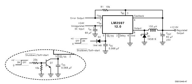
FIGURE 28. Typical Circuit Using Shutdown /Soft-start and Error Flag Features
