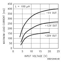
FIGURE 30. Maximum Load Current for Inverting Regulator Circuit
