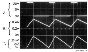
**Discontinuous Mode Switching Waveforms**  $V_{IN}$  = 20V,  $V_{OUT}$  = 5V,  $I_{LOAD}$  = 200 mA L = 33  $\mu$ H, C<sub>OUT</sub> = 220  $\mu$ F, C<sub>OUT</sub> ESR = 60 m $\Omega$
