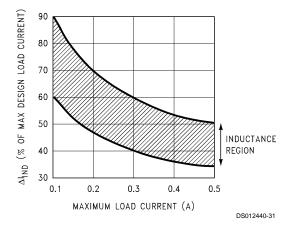
FIGURE 19. (△I<sub>IND</sub>) Peak-to-Peak Inductor Ripple Current (as a Percentage of the Load Current) vs Load Current
