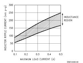
FIGURE 21. Peak-to-Peak Inductor Ripple Current vs Load Current
