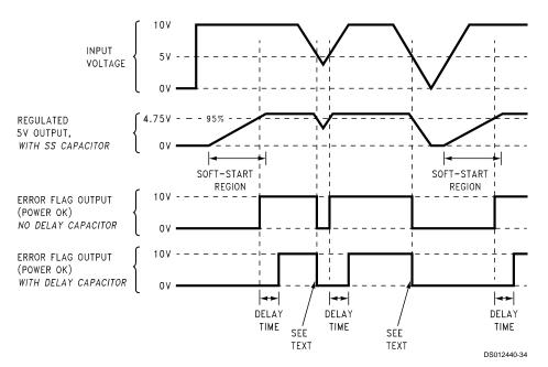
FIGURE 14. Timing Diagram for 5V Output
