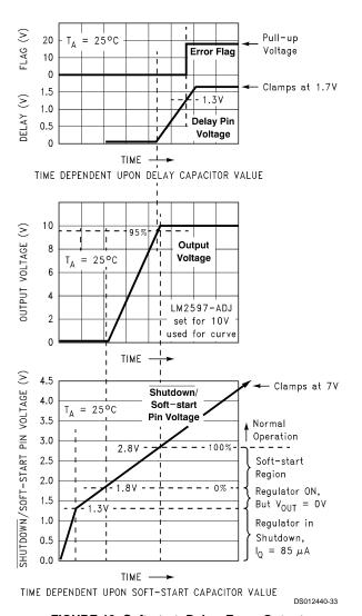
FIGURE 13. Soft-start, Delay, Error, Output
