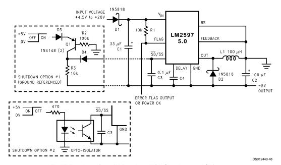
FIGURE 29. Inverting -5V Regulator With Shutdown and Soft-start
