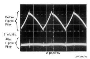
FIGURE 20. Post Ripple Filter Waveform
