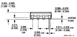
8-Lead (0.150" Wide) Molded Small Outline Package, Order Number LM2597M-3.3, LM2597M-5.0, LM2597M-12 or LM2597M-ADJ LM2597HVM-3.3, LM2597HVM-5.0, LM2597HVM-12 or LM2597HVM-ADJ NS Package Number M08A
