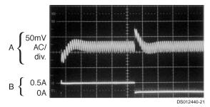
Load Transient Response for Discontinuous Mode  $V_{IN}$  = 20V,  $V_{OUT}$  = 5V,  $I_{LOAD}$  = 100 mA to 200 mA L = 33  $\mu\text{H},\,\text{C}_{\text{OUT}}$  = 220  $\mu\text{F},\,\text{C}_{\text{OUT}}$  ESR = 60  $\text{m}\Omega$
