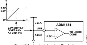
Figure 17. Setting the Undervoltage Threshold
