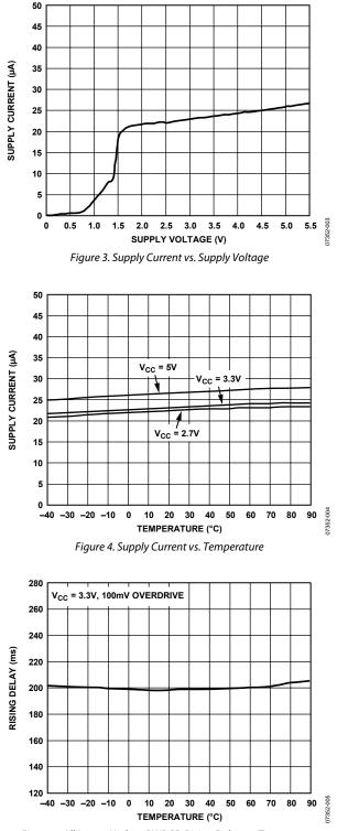
Figure 5. All Inputs High to PWRGD Rising Delay vs. Temperature
