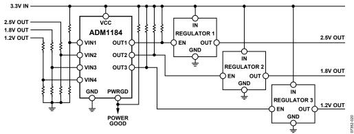
Figure 20. Voltage-Monitoring and Sequencing Application Diagram
