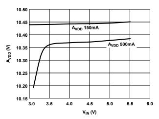
FIGURE 3. LINE REGULATION  $\mathbf{A}_{VDD}$  vs  $\mathbf{V}_{IN}$
