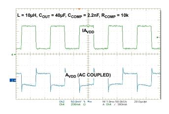
FIGURE 4. BOOST CONVERTER TRANSIENT RESPONSE
