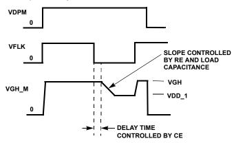
FIGURE 17. GATE PULSE MODULATOR TIMING DIAGRAM
