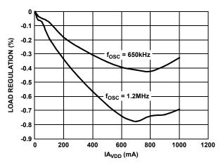
FIGURE 2.  $A_{VDD}$  LOAD REGULATION vs  $IA_{VDD}$
