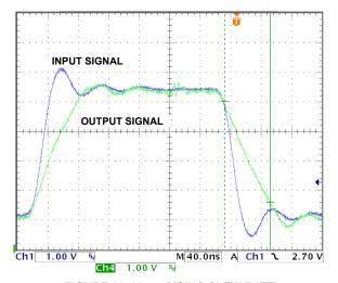
FIGURE 11.  $V_{\text{COM}}$  RISING SLEW RATE
