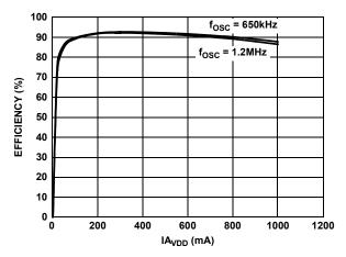
FIGURE 1.  $A_{VDD}$  EFFICIENCY vs  $IA_{VDD}$
