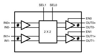
Figure 2. Block Diagram
