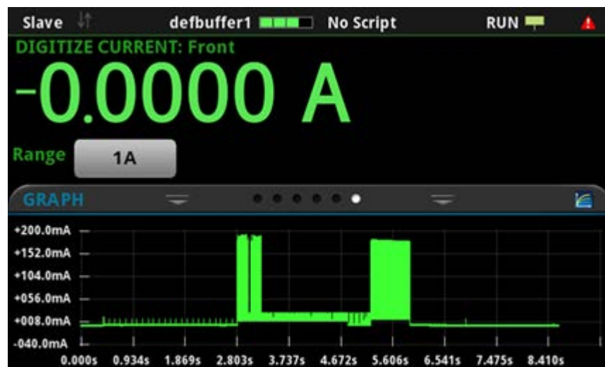
Figure 47: Subordinate node current waveform
