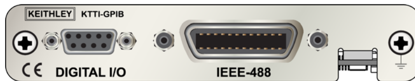
Figure 21: KTTI-GPIB connector view
