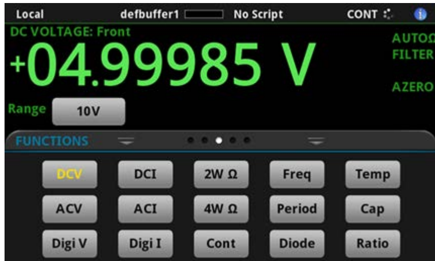
Figure 33: DC voltage high accuracy test results
