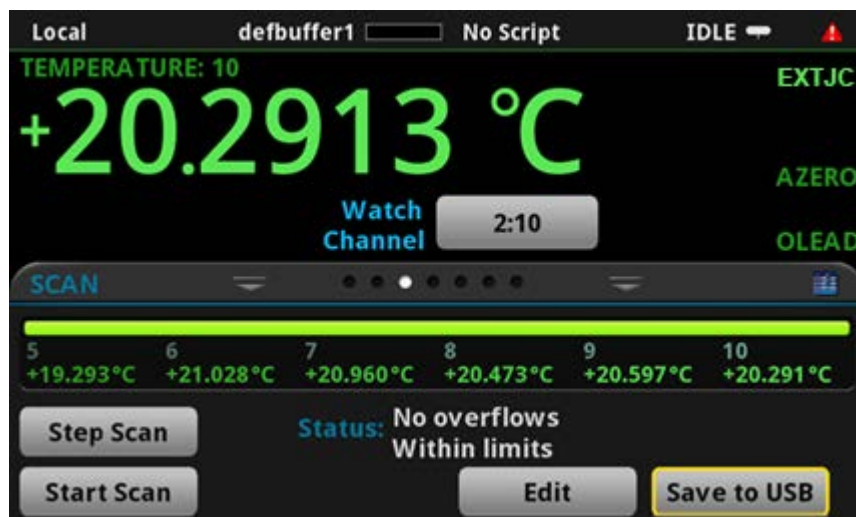
Figure 40: DMM6500 final temperature measurement
