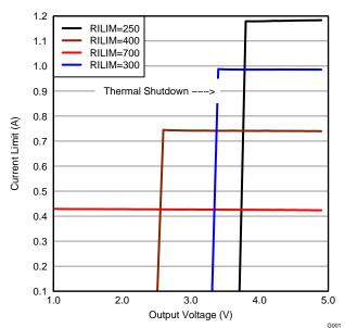
Figure 9. V<sub>OUT</sub> Sweep (I-V Curve)(2)
