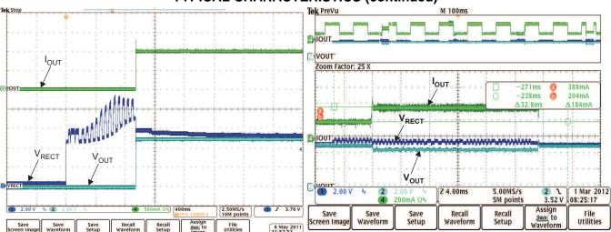
Figure 24. bq5101x Typical Startup with a 1A System Load
