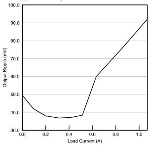
Figure 11. Output Ripple vs.  $I_{LOAD}$  ( $C_{OUT} = 1\mu F$ )
