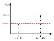
Figure 32. Termination Deglitch Timings for the CS100 Packet
