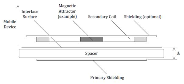
Figure 46. WPC v1.0 Receiver Coil Test Fixture for the Inductance Measurement Ls' (copied from System Description Wireless Power Transfer, volume 1: Low Power, Part 1 Interface Definition, Version 1.0.1, Figure 4-4)
