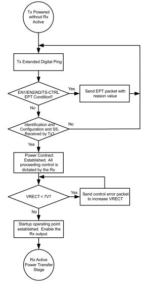
Figure 29. Wireless Power Startup Flow Diagram
