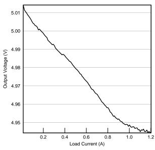
Figure 10. I<sub>LOAD</sub> Sweep (I-V Curve)
