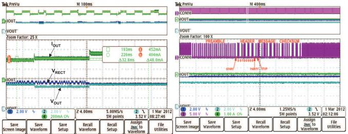
Figure 26. Adaptive Communication Limit Event Where the Current Limit is  $I_{OUT}$  + 50 mA ( $I_{OUT-DC}$  > 300 mA)
