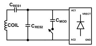
Figure 34. Capacitive Modulation
