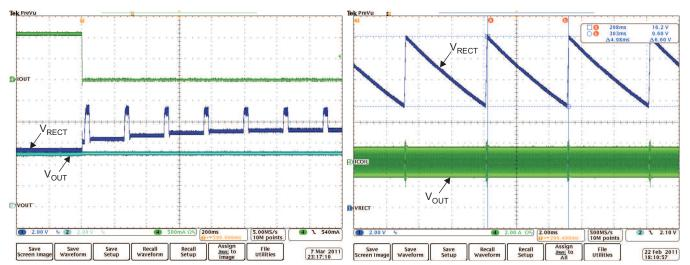
Figure 16. 1A Load Dump Full System Response
