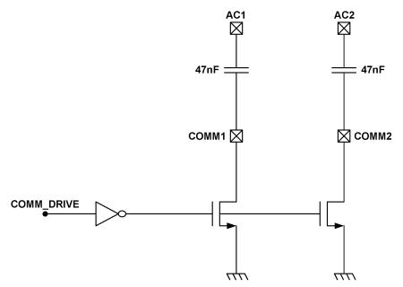
Figure 40. Capacitive Load Modulation
