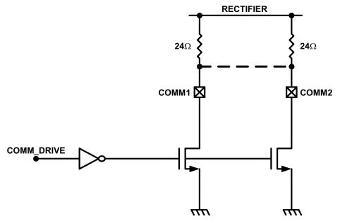
Figure 39. Resistive Load Modulation
