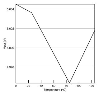
Figure 12.  $V_{OUT}$  vs Temperature
