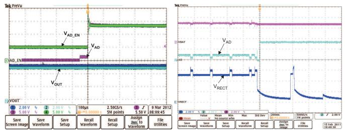
Figure 22. AD OVP Condition While Wireless Charging is Active (bq51014)
