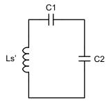
Figure 45. Dual Resonant Circuit with the Receiver Coil
