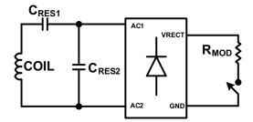
Figure 33. Resistive Modulation
