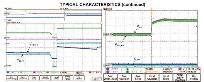
Figure 20. Adapter Insertion (V<sub>AD</sub> = 10V) Illustrating Break-Before-Make Operation
