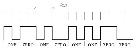
Figure 36. Differential Bi-phase Encoding Scheme (WPC volume 1: Low Power, Part 1 Interface Definition)
