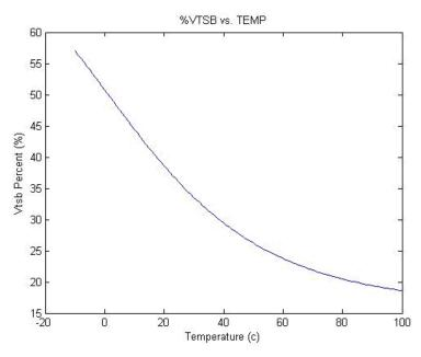
Figure 42. Example Solution for an NTC resistor with  $R_0 = 10K\Omega$  and  $\beta = 4500$
