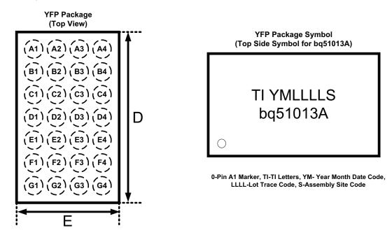
Figure 49. Chip Scale Packaging Dimensions
