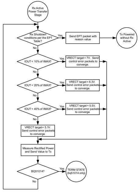
Figure 30. Active Power Transfer Flow Diagram
