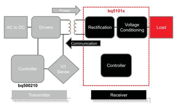
Figure 28. WPC Wireless Power System Indicating the Functional Integration of the bq5101x
