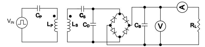
Figure 47. Load-Line Analysis Test Bench
