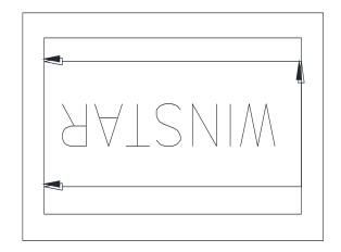
Fig. 1 Normal scan ( pin 4, LR/UD = High or NC )
