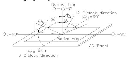
Fig.7.1. Definition of viewing angle
