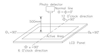
Fig. 7.2. Optical measurement system setup
