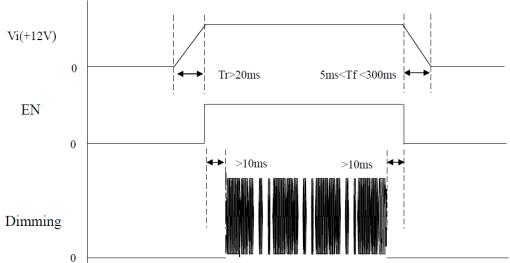
Note: While system is turned ON or OFF, the power sequences must follow as below descriptions Turn ON sequence:  $Vi(+12V) \rightarrow EN \rightarrow Dimming$  Turn OFF sequence: Dimming  $\rightarrow EN \rightarrow Vi(+12V)$
