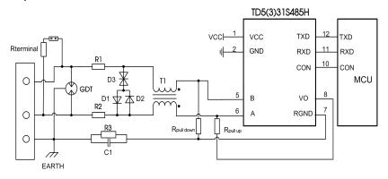
Fig. 2: Port protection circuit for harsh environments
