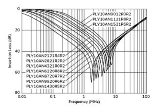
Differential Mode Insertion Loss-Frequency Characteristics
