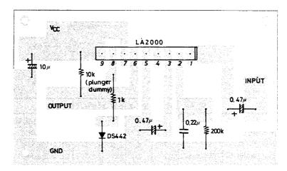
Unit (resistance:  $\Omega$ , capacitance: F)
