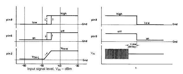
As shown above, when input level is raised and the pin 2 voltage reaches the  $V_{TH-H}$  level of the comparator, pins 6 and 8 turn over. ( $V_{IN} = -45 \text{ dBm}$ ).
