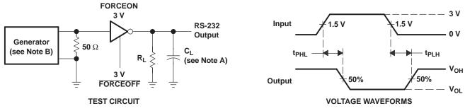
NOTES: A. C<sub>L</sub> includes probe and jig capacitance. B. The pulse generator has the following characteristics: PRR = 250 kbit/s,  $Z_O = 50 \Omega$ , 50% duty cycle,  $t_f \le 10$  ns.  $t_f \le 10$  ns.
