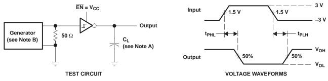
NOTES: A. C<sub>L</sub> includes probe and jig capacitance. B. The pulse generator has the following characteristics:  $Z_O = 50 \ \Omega$ , 50% duty cycle,  $t_r \le 10 \text{ ns}$ .
