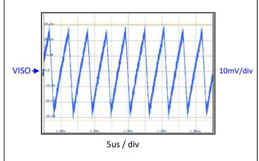
Figure 7- 11.  $V_{INP} = 5V$ ,  $V_{ISO} = 3.3V$ ,  $I_{ISO} = 130mA$ ;
