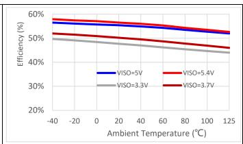
Figure 7- 26. Power Supply Efficiency vs. Temperature
