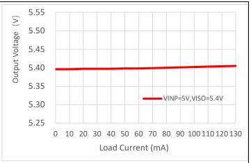
Figure 7- 18. V<sub>ISO</sub> Load Regulation; V<sub>INP</sub> = 5V, V<sub>ISO</sub> = 5.4V
