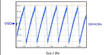
Figure 7- 10  $V_{INP} = 5V$ ,  $V_{ISO} = 5.4V$ ,  $I_{ISO} = 130$ mA;
