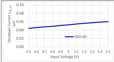
Figure 7- 27. Shutdown Current vs. Input voltage;
