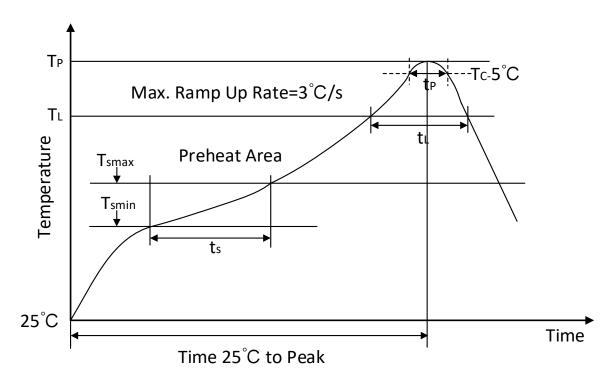
Figure 11-1 Soldering Temperature (reflow) Profile
