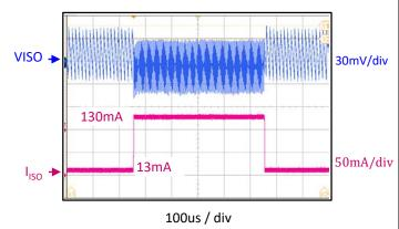
Figure 7- 14. V<sub>ISO</sub> Load transient response V<sub>INP</sub> = 5V, V<sub>ISO</sub> = 5.4V, Load step: 13mA to 130mA; V<sub>ISO</sub> ripple voltage(peak to peak): 17mV
