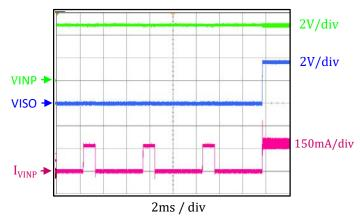
Figure 7-8.  $V_{INP}$  = 5V,  $V_{ISO}$  = 3.7V, output short to GNDS and recover to I<sub>ISO</sub> = 130mA
