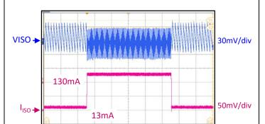
Figure 7- 15.  $V_{ISO}$  Load transient response:  $V_{INP}$  = 5V,  $V_{ISO}$  = 3.3V, Load step: 13mA to 130mA;  $V_{ISO}$  ripple voltage(peak to peak): 15mV
