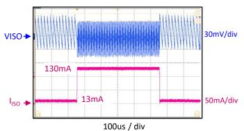
Figure 7- 16.  $V_{ISO}$  Load transient response:  $V_{INP}$  = 5V,  $V_{ISO}$  = 3.7V, Load step: 13mA to 130mA;  $V_{ISO}$  ripple voltage(peak to peak): 16mV
