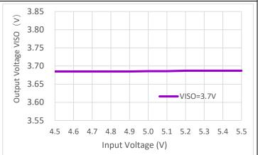
Figure 7- 23.  $V_{\text{ISO}}$  Line Regulation;  $V_{\text{INP}}$  = 4.5V to 5V,  $V_{\text{ISO}}$  = 3.3V
