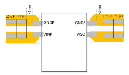
Figure 9-2. Recommended Bypass Capacitors Placement
