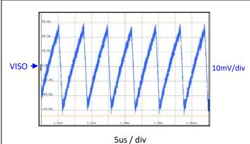
Figure 7- 9.  $V_{INP} = 5V$ ,  $V_{ISO} = 5V$ ,  $I_{ISO} = 130$ mA;
