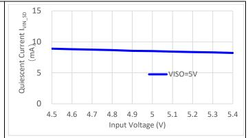
Figure 7- 28. Quiescent Current vs. Input Voltage V<sub>INP</sub> = 4.5V to 5.5V, V<sub>ISO</sub> = 5V, EN connected to VINP
