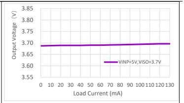
Figure 7- 19. V<sub>ISO</sub> Load Regulation; V<sub>INP</sub> = 5V, V<sub>ISO</sub> = 3.3V
