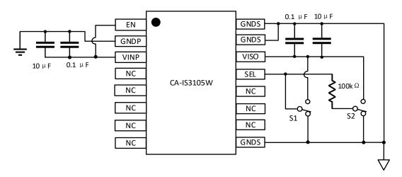
Figure 9-1. CA-IS3105W Typical Application Circuit
