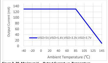
Figure 7- 29. Maximum V<sub>ISO</sub> Output Current vs. Temperature ,
