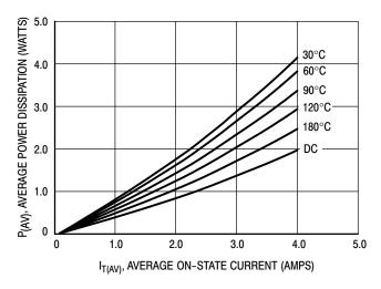
Figure 2. On-State Power Dissipation
