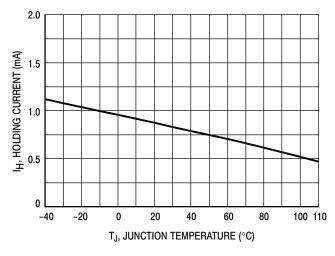
Figure 7. Typical Holding Current versus Junction Temperature
