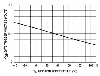
Figure 6. Typical Gate Trigger Voltage versus
