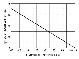
Figure 5. Typical Gate Trigger Current versus Junction Temperature
