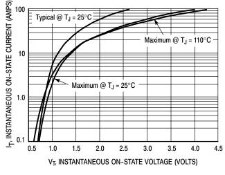
Figure 3. On-State Characteristics
