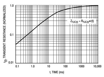
**Figure 4. Transient Thermal Response**
